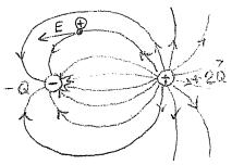
In this case, the number of lines that leave the positive charge +2q is twice the number entering the charge -q. Hence only half that leave the positive charge enter the negative charge, leaving the remaining half terminate on a negative charge we assume to be located at infinity.
