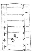
Notice, that the electric field lines are perpendicular to the plates, parallel to each other and uniform or equally spaced, except near the edges. This indicates that the electric field strength is constant between the two plates.
